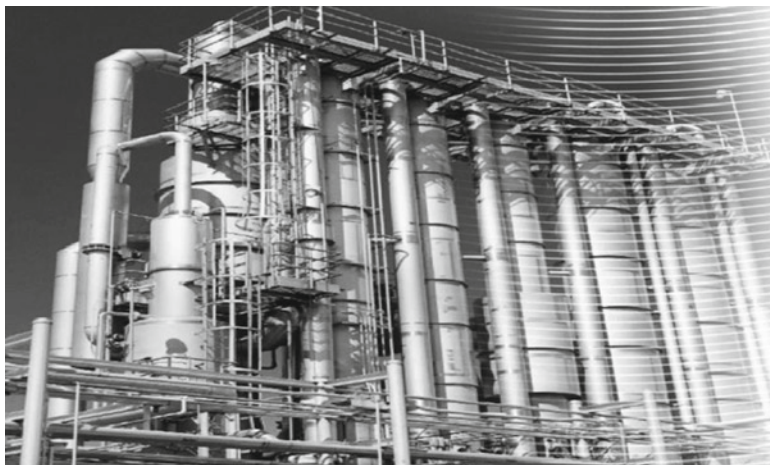
Fig. 6 Falling film evaporator (Courtesy: Niro Inc.)
