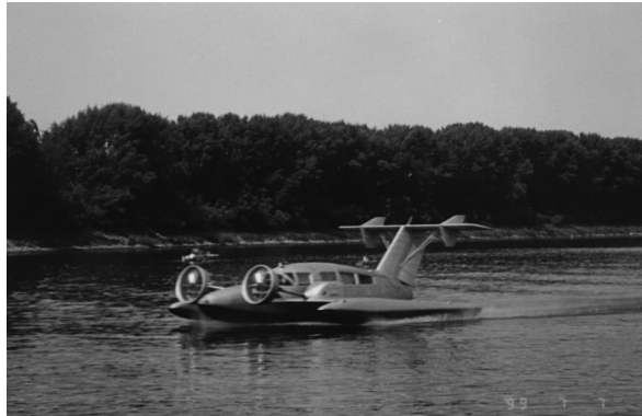
Fig. 2.27 Dynamic air cushion craft (DACC) type “Volga-2”
