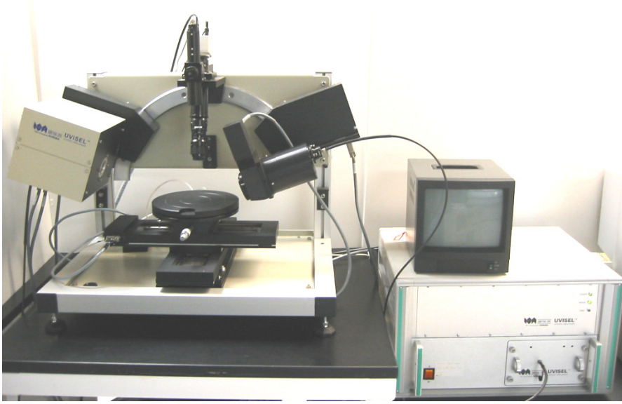
Fig. 2.6. A typical ellipsometer system, including a light source and its power supply, a sample stage, a detector and the analyzing circuits.
