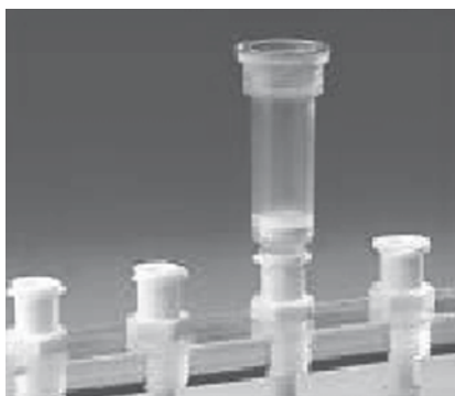
Fig. 1. Standard configuration for a vacuum manifold system fitted with RNeasy microcolumns. This approach allows the processing of large volumes of RNA extraction buffer (e.g., >5 ml) through the silica membrane without the use of a centrifuge.
