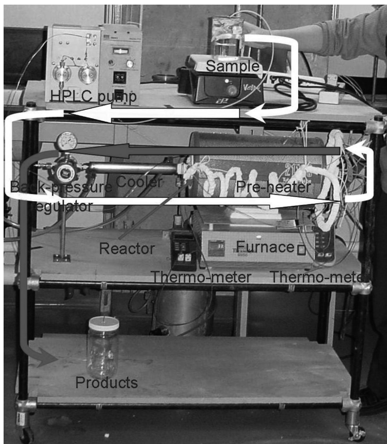
Fig. 2.11 Image of the flow reactor built in our lab
