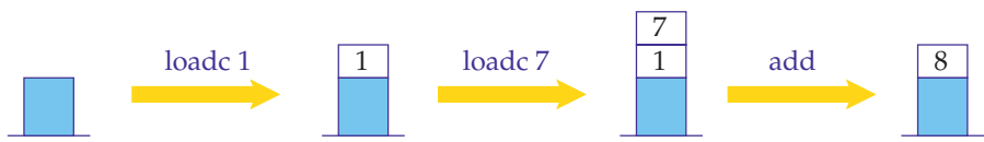
Fig. 2.6. Executing the instruction sequence for 1 + 7
