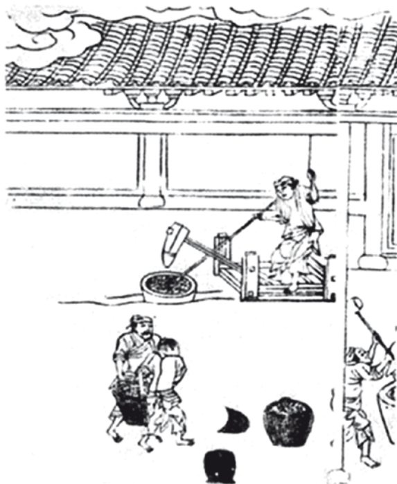
Fig. 2.10 Foot-operated hammer (From the Kêng Chih Thu [86])
