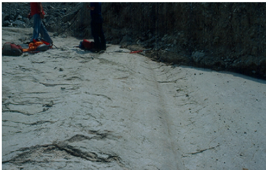
Figure 2.9 A striated continuous clay layer belonging to the sliding surface (courtesy of G. Fernández).
