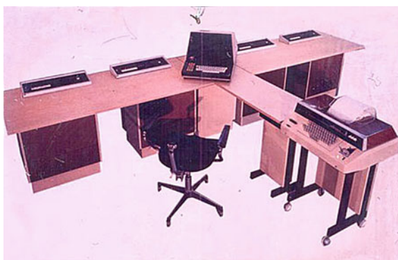
Fig. 2.3 DEMP—decentralized, modular, multiprocessor—high reliability computer architecture
