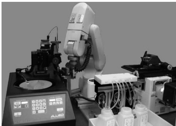
Fig. 5 The automated serial sectioning device RoboMet3.D (Spowart et al. 2003; Spowart 2006). From left-to-right in the image are the precision metallographic polisher, six-axis robot, etching/washing/drying station, and a motorized inverted optical microscope. Figure is used with permission from Elsevier
