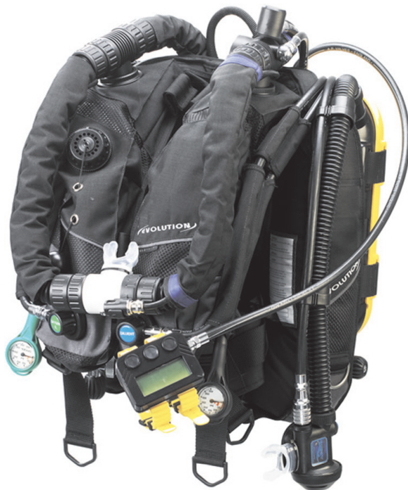
Figure 2.9. The Evolution showing the harness, wings, and hose. The system is an electronics-driven fully closed-circuit constant partial pressure of oxygen rebreather that provides the diver with a host of diving information via a heads-up display. It costs about US$10,000. Photo John Bantin. Courtesy Ambient Pressure Diving.
