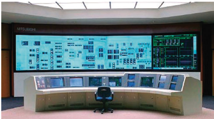
Fig. 2.4 Advanced main control board (prototype)
