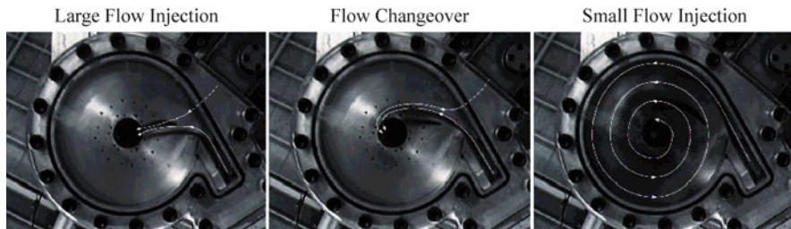
Fig. 2.34 Visualized flows in the vortex chamber of the 1/5-scale model are shown. White lines are added as guides to indicate the observed flow directions. There was no vortex for the large flow injection, while a strong and steady vortex was formed for the small flow injection. The change-over of the flow from the large to small flow injections was quick and continuous
