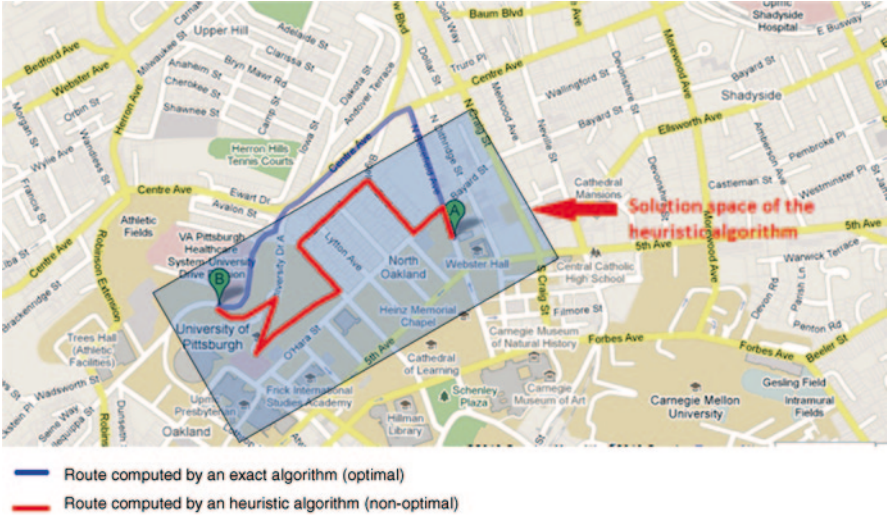
Fig. 2.12 An optimal route computed by an exact algorithm and a non-optimal route computed by a heuristic algorithm
