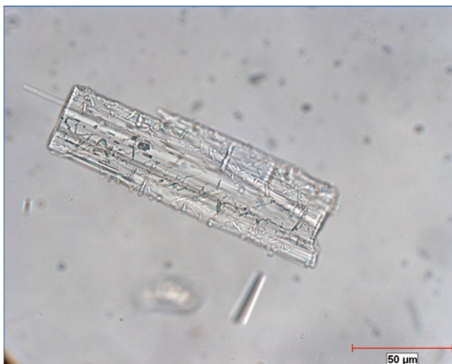
Fig. 2.10 Caffeine Form II growing on crystal of Form I. Appearance of crystals growing on the surface of the original crystals is one good application of assessment of surface texture during stability trials. (Image size=210×170 μm)
