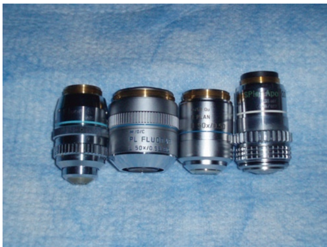
Fig. 2.25 Microscope objectives. From left to right, Nikon 40x/0.85 NA 160 mm tube length fluorite objective; a Leitz reflected light 50x/0.55 NA fluorite infinity-corrected objective; a Leica 50x/0.50 NA achromat infinity-corrected objective, an Olympus 100x/1.35 NA apochromat oil immersion 160 mm tube length objective
