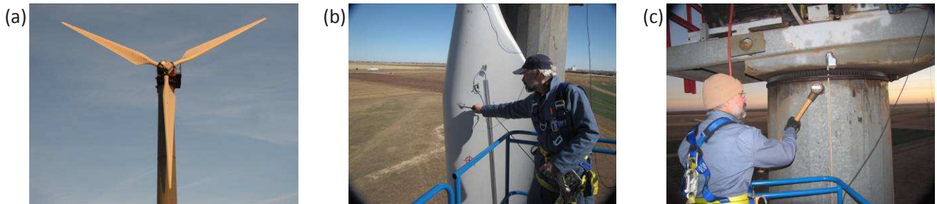
Figure 4: (a) Micon 65/13 Wind Turbine with the Sensed Rotor Blade mounted. (b) Modal impact testing of the wind turbine rotor blades. (c) Modal impact testing of the wind turbine tower.
