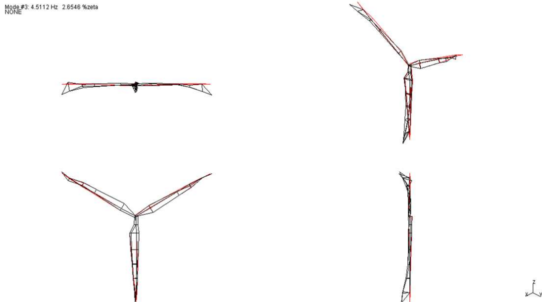
Figure 5: 1 st Umbrella Mode Shape of rotor plane from modal test experiment.
