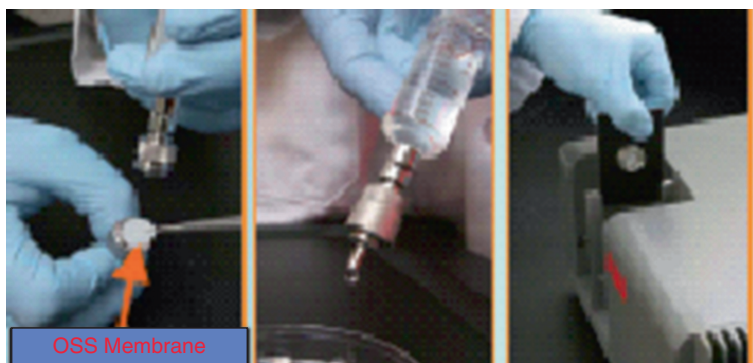
Fig. 2.5 Pictures showing the steps involved in the OSS solventless IR technology (Martin et al. 2008)
