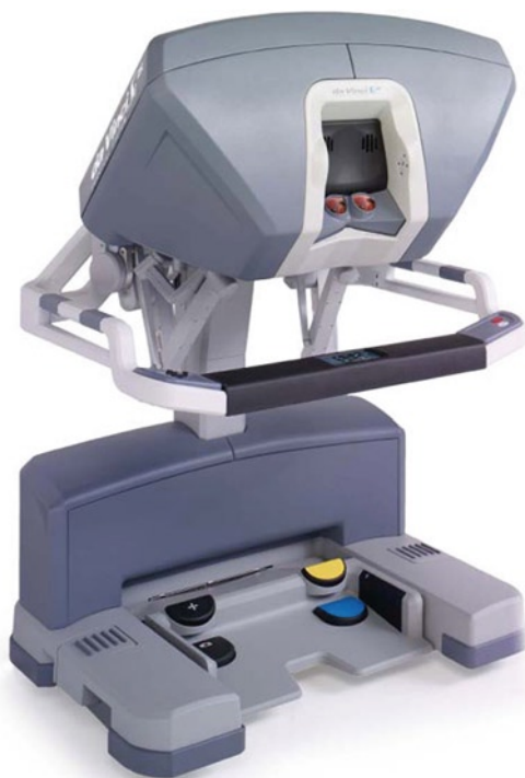
Fig. 2.7 Photograph of da Vinci® Si-HD surgeon console (Reproduced with permission from Intuitive Surgical, Inc © 2009)
