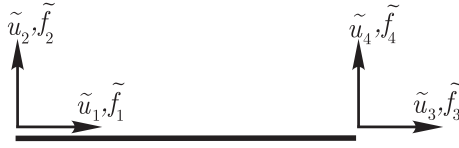
Fig. 2.23. Degrees of freedom of a truss bar
