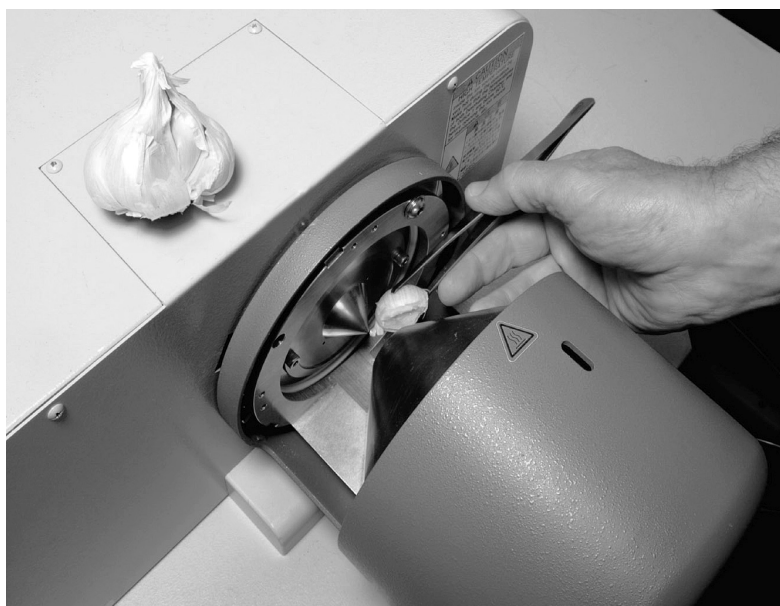
Fig. 13.19. Commercial DART source. Here it is used for the analysis of volatiles from a garlic clove. The sample is simply held in the open gap between the metastable atom source ( lower right part ) and the orifice of the API interface ( upper left ). Photograph by courtesy of JEOL USA.
