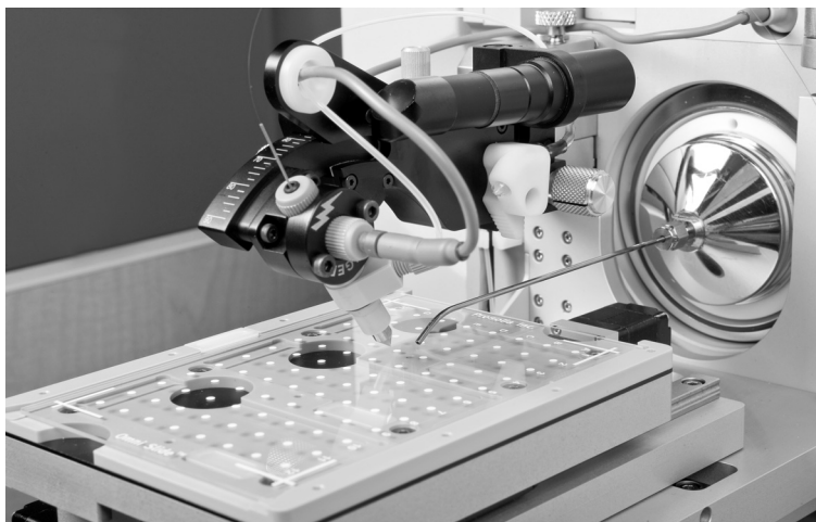
Fig. 13.4. A commercial DESI ion source. This one here is the Prosolia Omni Spray 2D source coupled to a Thermo Fisher LTQ mass spectrometer. The surface shown is a 96-spot Omni Slide HC having the standard microtiter plate dimensions. Note the extended desolvation capillary and the adjustable sprayer. Courtesy Prosolia, Inc., Indianapolis, In USA.
