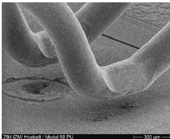
Fig. 11.44 Lifted bond wires after power cycling test with \Delta T_j = 100 K of a standard IGBT module. The total failure occurred between 10,791 and 13,000 cycles
