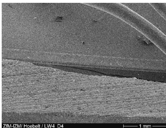
Fig. 11.55 Crack in the silicon diode chip in a transfer mold TO package on a Cu-lead frame after 3800 cycles with \Delta T_j = 110 K and T_m = 95^\circ\text{C}
