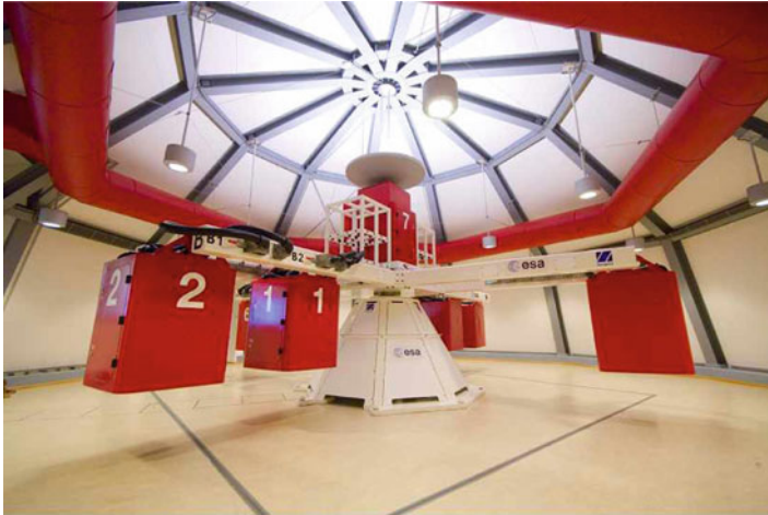
Fig. 2.20 The ESA Large Diameter Centrifuge (LDC) at ESA-ESTEC, Noordwijk, the Netherlands (Source: ESA)
