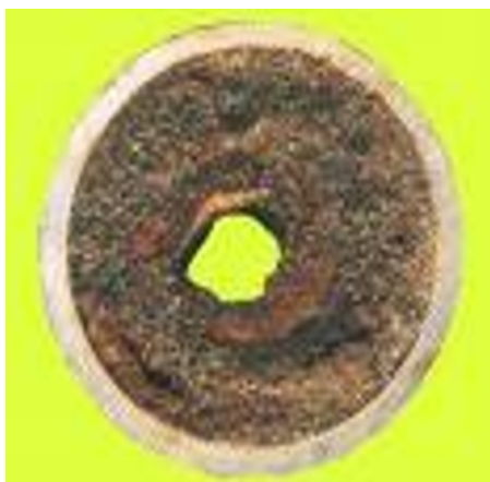
Figure 1. Section of a pipeline with deposited wax
