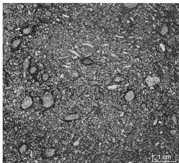
Horticulture Substrates, Structure and Physical Properties, Figure 1 Structure of the mixture of white peat (50%, v/v) with coconut fiber (50%, v/v). Image in 256 gray degrees of polished opaque block (surface dimensions 8 × 9 cm) developed from this substrate impregnated with polyester resin. Color of the pores is black and of the solid phase – gray (Słowińska-Jurkiewicz and Jaroszuk-Sierocińska, 2007).
