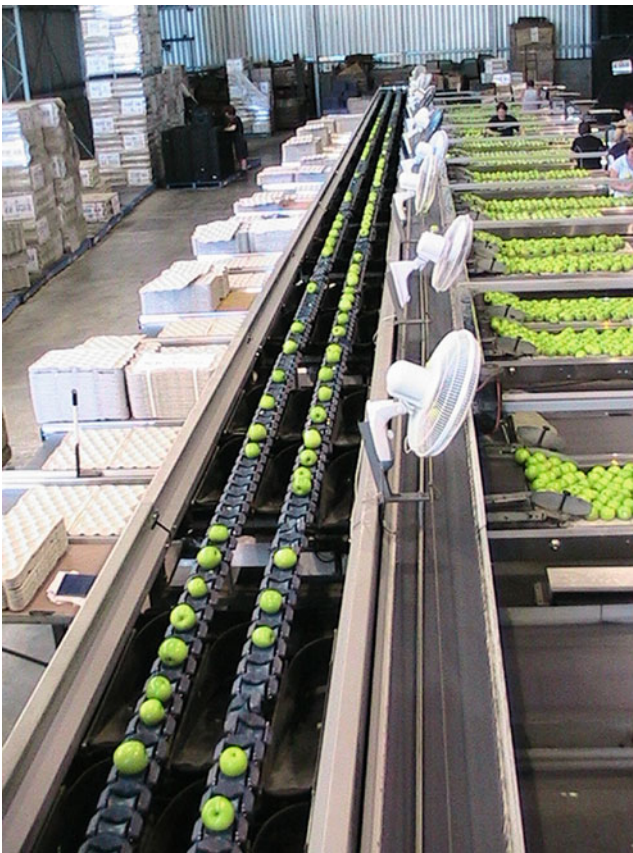
Machine Vision in Agriculture, Figure 2 A conveyor automatically ejects each apple at the correct station.
