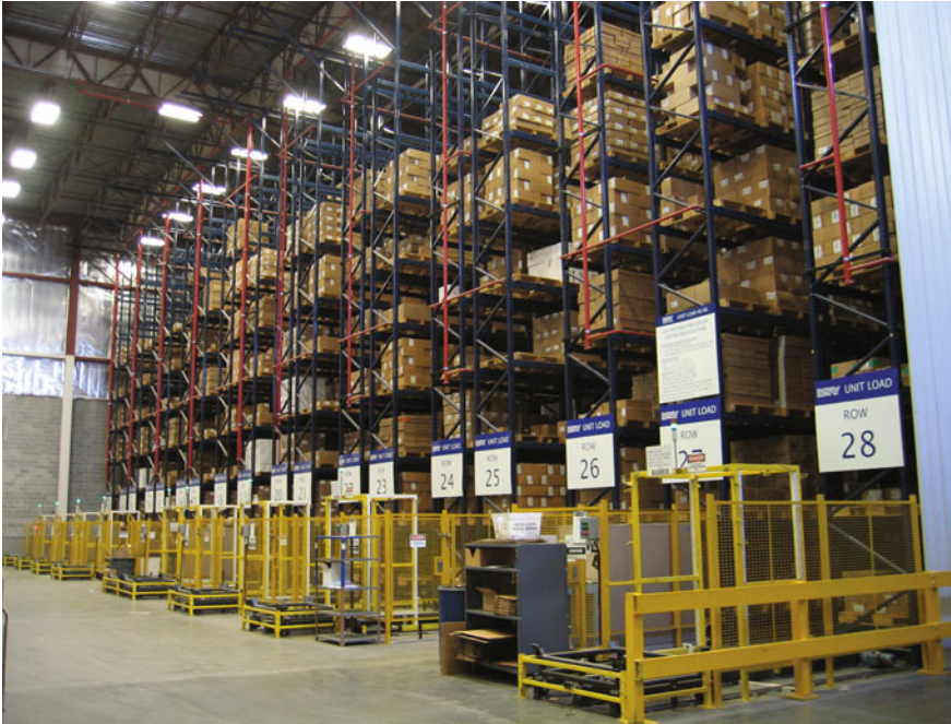
Fig. 2.2 Parallel aisles of a pallet rack (photos courtesy of LogisticsCAD, used with permission)
