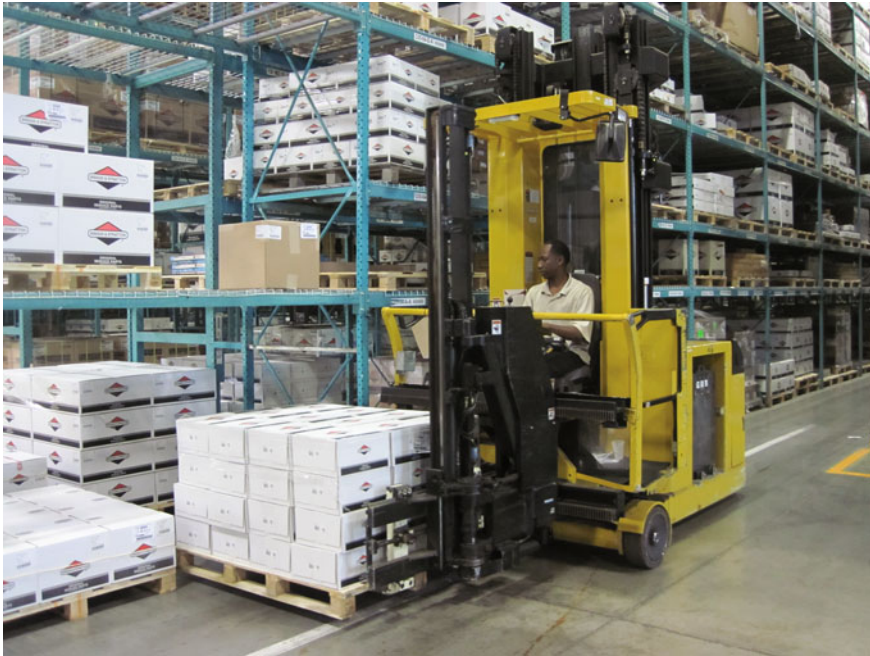
Fig. 2.3 Turret truck accessing a unit load (photo courtesy of LogisticsCAD, used with permission)
