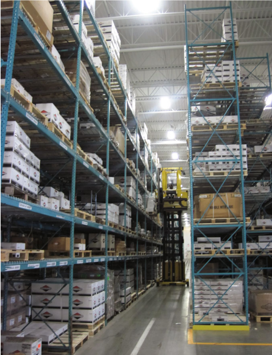
Fig. 2.1 Single-deep pallet rack (photos courtesy of LogisticsCAD, used with permission)
