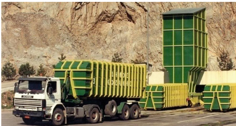
Fig. 3 Transfer station with a hopper, a compactor unit and semitrailers for the transportation of containers
