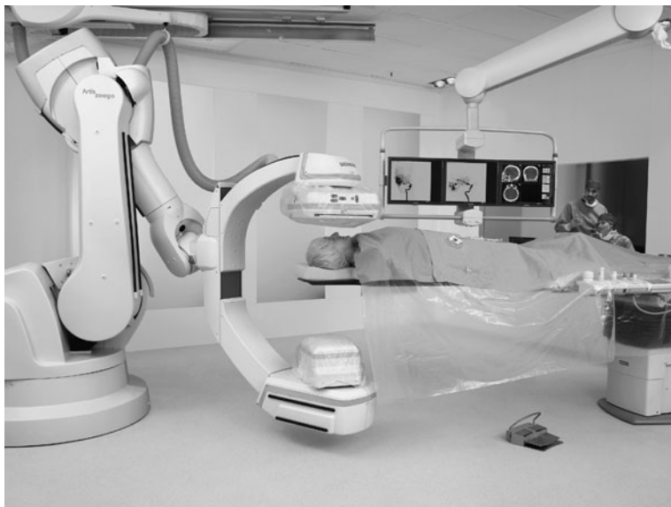
Fig. 2.11 Angiographic imaging device (C-arm) which is used for guiding minimal invasive interventions (Siemens Artis zeego, with kind permission from Siemens Sector Healthcare, Erlangen, Germany)
