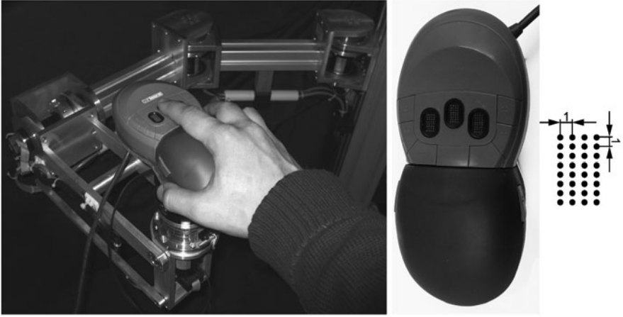
Fig. 2.9 Left: Kinesthetic device (DeKIFeD 4) in combination with the tactile device (VirTouch Mouse). Right: Close-up view of the VirTouch Mouse containing three Braille modules and proportions of the Braille module. Distances are in millimeters
