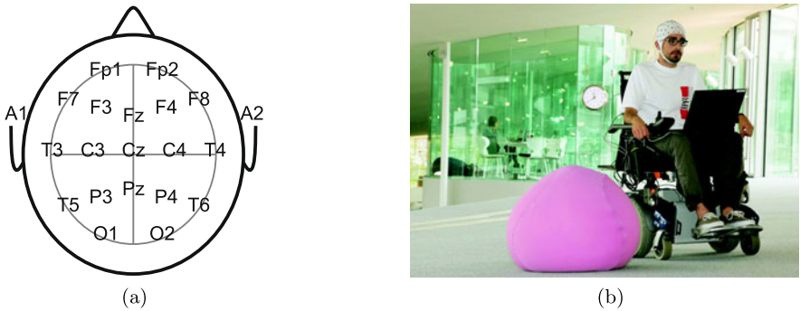
Fig. 2.14 Electroencephalographic (EEG) methods: (a) International 10-20 system of electrode placement [11], (b) EEG-based brain-computer interface; by courtesy of Dr. José del R. Millán
