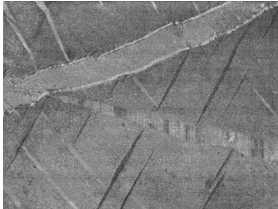
Fig. 2.3 The structure of a \text{ZrH}_{1.27} specimen showing banded \gamma -hydride precipitates in a \delta -hydride matrix and a third phase at the grain boundary (from Barraclough and Beevers [5])
