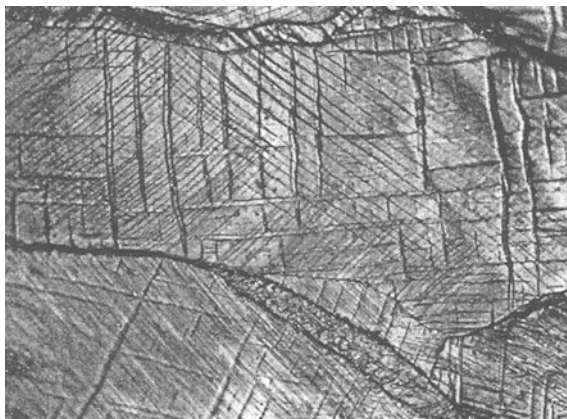
Fig. 2.14 Large distorted \gamma -hydride platelets in a \text{ZrH}_{1.27} specimen after 11 % strain (from Barraclough and Beevers [3])
