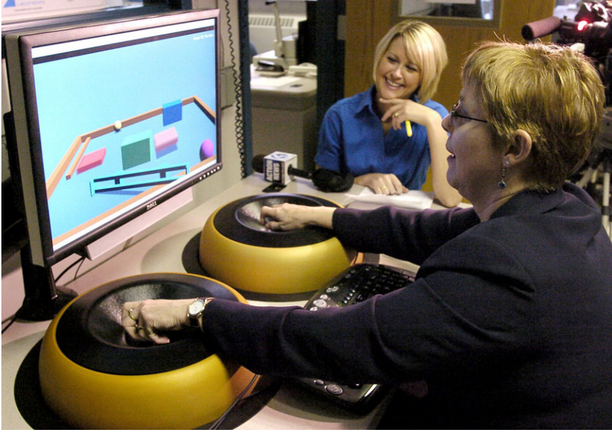
Fig. 2.8 Maglev 200™ Magnetic Levitation Haptic Interface is the first commercial haptic device to employ the principles of Lorentz levitation. The handle can be freely moved in 6 DOF with zero friction. Photo courtesy of Butterfly Haptics, LLC
