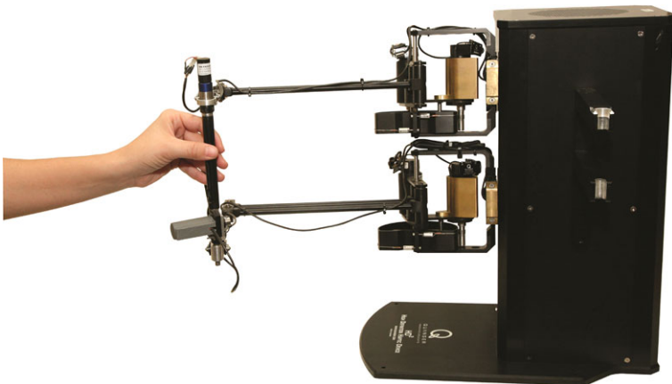
Fig. 2.7 The 6 DOF High Definition Haptic Device (HD 2 ), developed by Quanser Inc., is a high fidelity force-feedback platform for advanced research in haptics and robotics. Photo courtesy of Quanser Inc.
