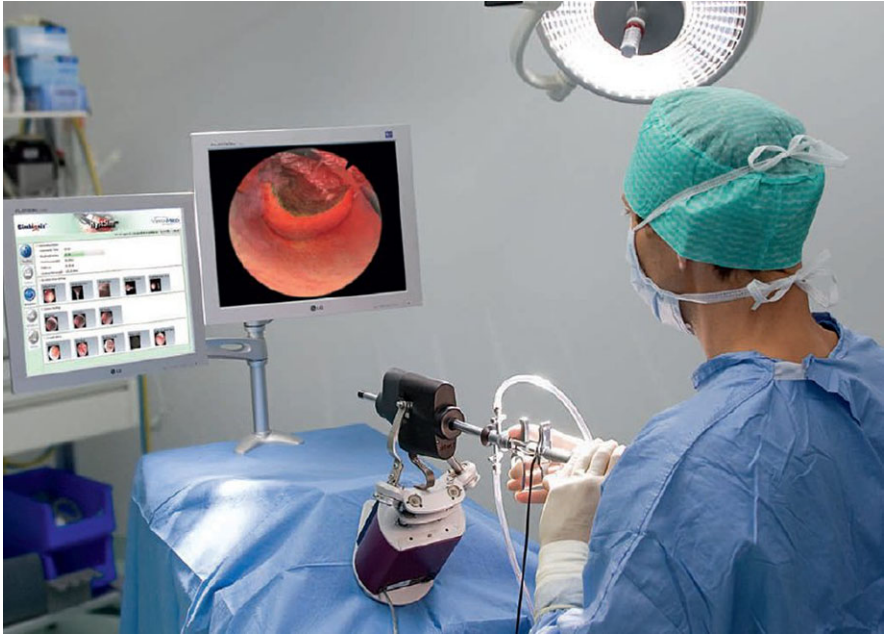
Fig. 2.10 VirtaMed HystSim system employing the Xitact™ IHP as the force feedback interface. Photo courtesy of VirtaMed AG
