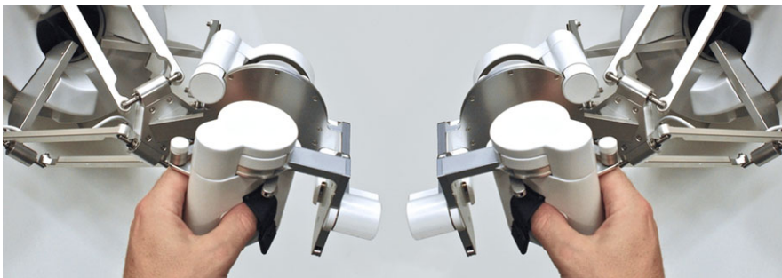
Fig. 2.4 The sigma.7 haptic device from Force Dimension. Being the most advanced haptic interface developed by Force Dimension, it introduces 7 active DOFs, including grasping capability. Photo courtesy of Force Dimension
