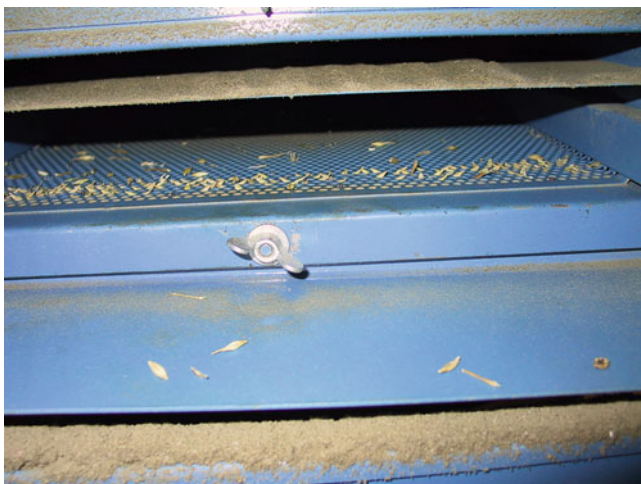
Fig. 2.5 Sieve for the separation of foreign matter from oilseeds
