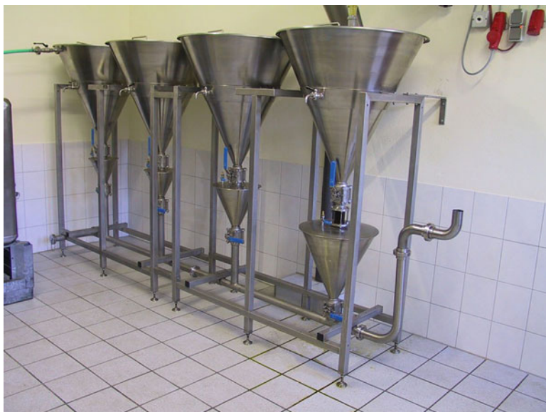
Fig. 2.17 Multilevel sedimentation system for the purification of rapeseed oil (by courtesy of Technologie und Förderzentrum, Straubing, Germany)
