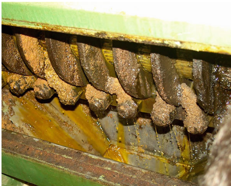
Fig. 2.8 Barrel of a screw press surrounded by flat bars during pressing of oilseeds
