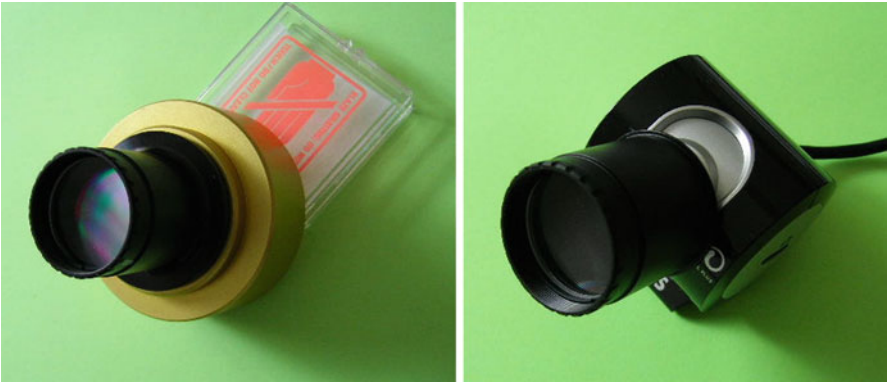
Fig. 2.2 Filter gratings fitted to a QHY5 camera and Philips SPC900 webcam
