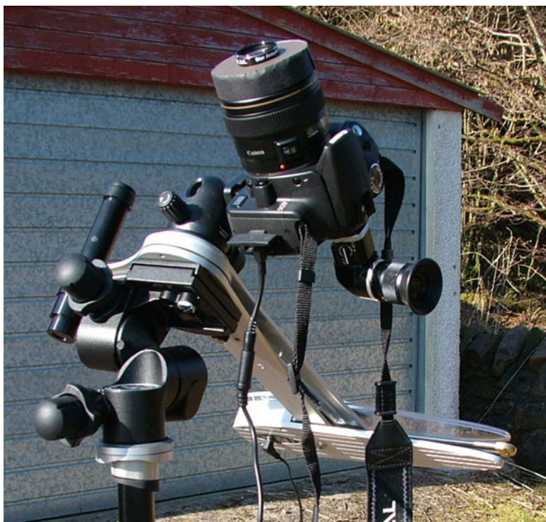
Fig. 2.10 SA100 objective grating mounted on 85 mm telephoto lens (J. Simpson)
