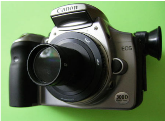
Fig. 2.3 Filter grating fitted to a Canon 300D DSLR
