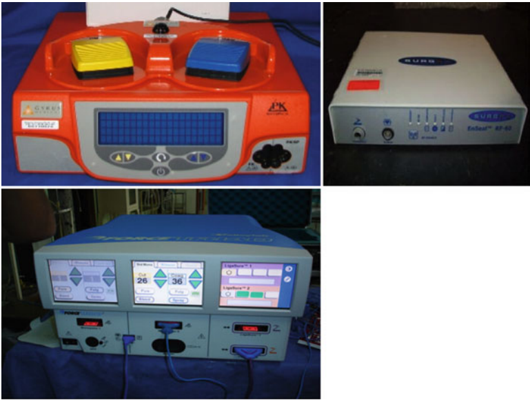
Fig. 2.10. Proprietary electrosurgical units. Depicted are three ESUs designed to run proprietary bipolar systems: The PlasmaKinetic system (Olympus-Gyrus, Inc.), upper left ; the EnSeal system (Ethicon Endosurgery, Inc.), upper right ; and the Force Triad that supports the LigaSure system (Covidien, Inc.), lower left . There are a number of different ESU's on the market that are designed to support proprietary bipolar instruments.
