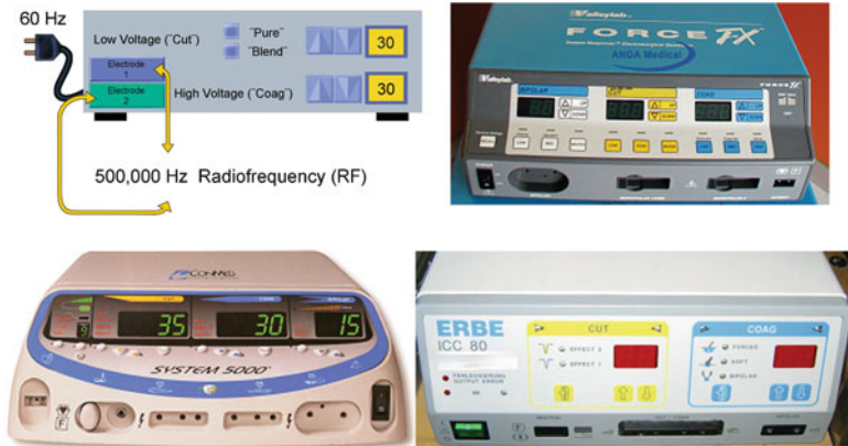
Fig. 2.7. A stylized electrocautery unit (ESU) is depicted in the upper left . It converts alternating current from a wall source (50–60 Hz), to a radiofrequency output, typically about 500 KHz (500,000 Hz). The circuit is formed using two outlets. The three commercial examples shown each have similar colors for waveforms used for monopolar instrumentation—a low-voltage (“cut”) output coded in yellow and a modulated high-voltage output (“coag”) coded in blue . The “Force FX” ( upper right ) and the “System 5000” ( lower left ) each have a bipolar output that is coded in blue , even though the bipolar outputs are low voltage, similar to those of the yellow-coded “cut” outputs.
