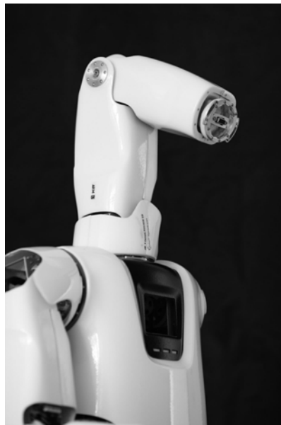
Fig. 2.8 All body parts of the robot MYON can be detached and reattached during runtime. Here, the head has been replaced by the robot's left arm.
