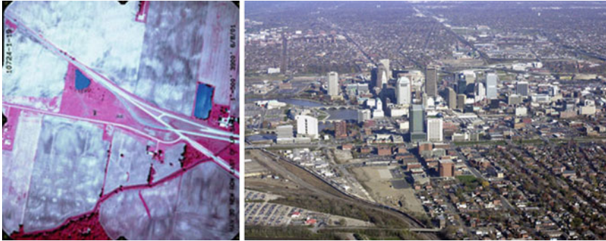
Fig. 2.3 A vertical aerial photograph ( left ) and an oblique aerial photograph ( right ). Images courtesy of Ohio Department of Transportation
