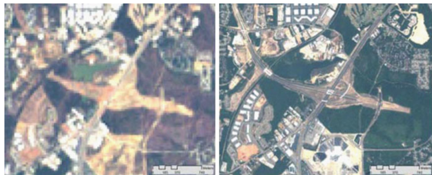
Fig. 2.1 Landsat ETM+ ( left ) and Quickbird ( right ) images of the same area, demonstrating the large difference in spatial resolution between the two sensors (Landsat ETM+ multispectral resolution = 30 m; Quickbird multispectral resolution = 2.62 m). In the Quickbird image, individual buildings and minor road features are readily discernible
