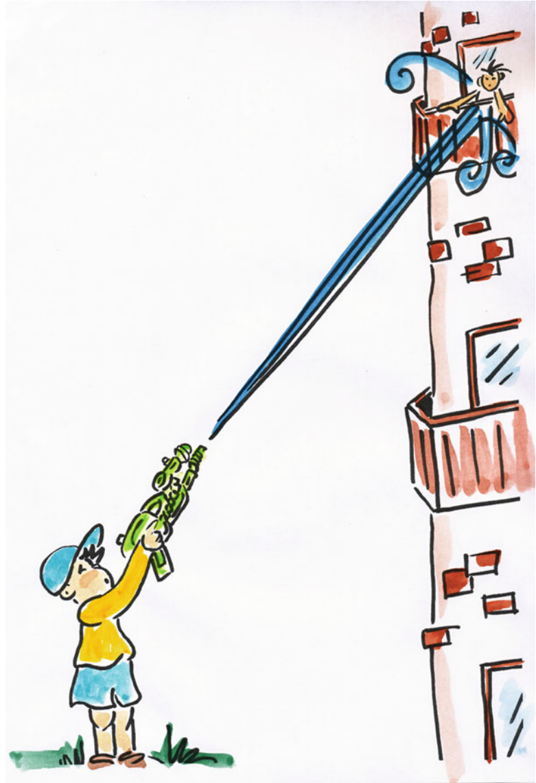
Fig. 2.3 High voltage (analogous to the high water pressure) allows arcing through the air
