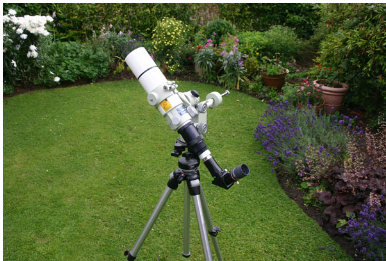
Fig. 2.3 The author's 60 mm (2.4 in.) f/5.9 Takahashi apochromatic refractor. Its short tube makes it extremely compact and portable
