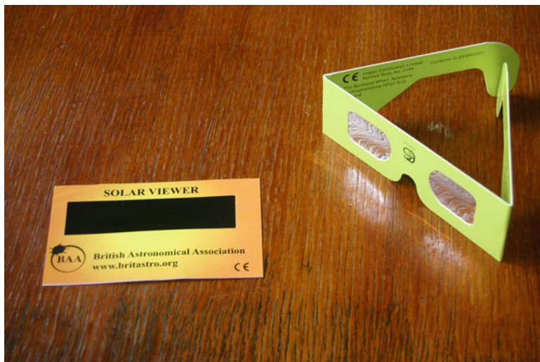
Fig. 2.11 A naked-eye solar viewer made from black polymer ( left ) and a pair of Mylar eclipse glasses ( right )
