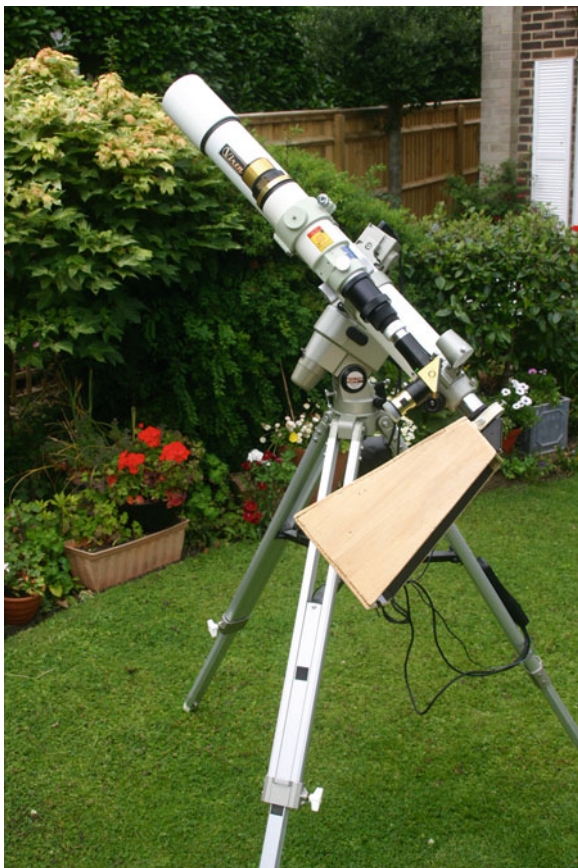
Fig. 2.2 The author's 80 mm (3.1 in.) refracting telescope on a German equatorial mount with electronic slow motion controls. A home-made balsa wood projection box is attached to the eyepiece end of the telescope for safe viewing of the Sun's image
