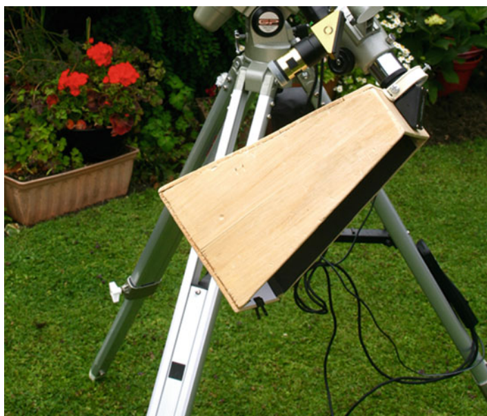
Fig. 2.7 A balsa wood projection box made by the author and attached to an 80 mm (3.1-in.) refractor
