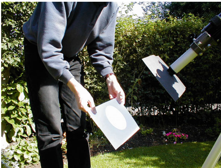
Fig. 2.5 Projecting the Sun's image onto paper for safe solar viewing. A card has been fitted over the eyepiece end of the telescope to shade the image from direct sunlight
