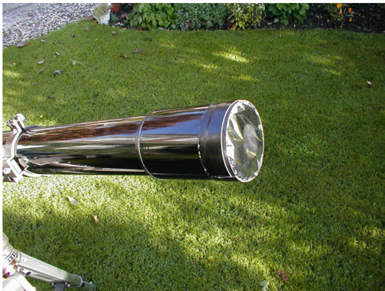
Fig. 2.8 Aperture filter made from Baader AstroSolar Safety Film in a home-made mount, fitted to an 80 mm refractor
