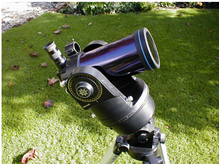
Fig. 2.4 A Meade ETX 90 mm (3.5 in.) Maksutov telescope equipped with a glass aperture filter. Note that the finderscope has been removed. This is an important safety precaution, because the Sun is just as dangerous to look at through the finderscope as the main telescope, and careless people, particularly children, could look through it by accident
