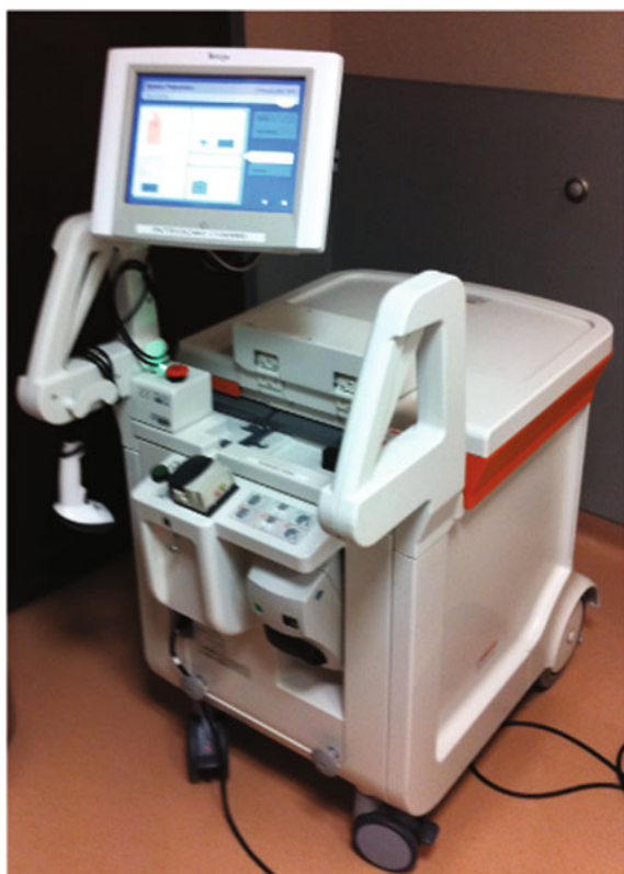
Fig. 2 This is an example of a mobile FDG administration device. From the shielded multidose vial within the machine, the individual patient's FDG activity is measured and administered. FDG dosing is controlled via computer to provide efficient delivery consistently within 2 % of the requested amount
