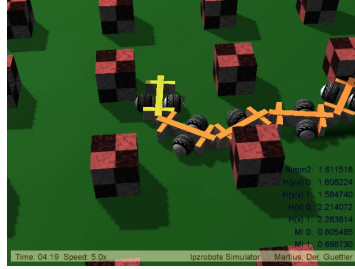
Video 3.4: The chain of robots with decentralized control in a regular maze. Spontaneous cooperativity and sensitive reactions to collisions helps the chain to navigate in the maze without any proximity sensors. The video can be watched at http://playfulmachines.com .
