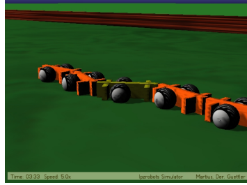
Video 3.3: Emerging cooperativity in a chain of TwoWHEELS. The arena has no obstacles. Control is completely decentralized, but the individual wheels spontaneously cooperate in the working regime close to the effective bifurcation point. The video can be watched at http://playfulmachines.com .
