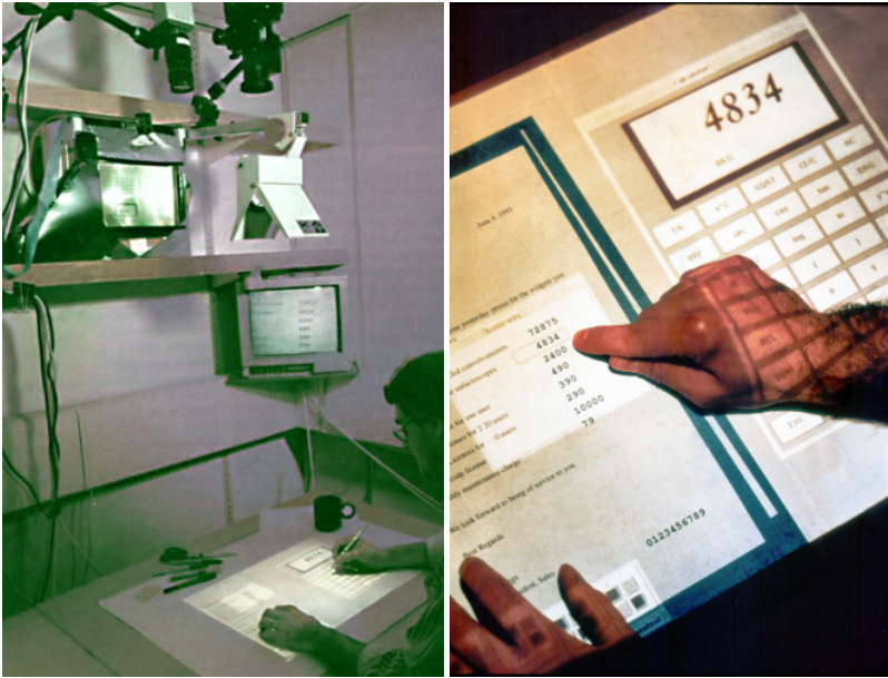
Fig. 2.21 The DigitalDesk. Left: Tracking-projection setup of the prototype. Right: copy&paste between a paper document and a calculator application (photos courtesy of Pierre Wellner)
