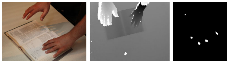
Fig. 2.4 Detecting touch using a depth camera. Left: Touching a book. Center: Depth image. Right: Detected contacts (photos courtesy of Andy Wilson)
