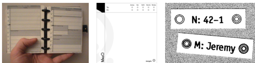
Fig. 2.12 The PaperPDA. Center: A form for writing e-mails on paper. Right: Physical stickers for creating hyperlinks (photo courtesy of Scott Hudson)
