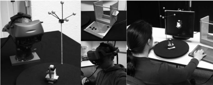
Fig. 6.126 Experiment configuration with turntable and HMD ( left ), experiment configuration with monitor ( right ), keypad for manipulating the virtual object ( top centre ), participant wearing the HMD ( bottom centre )
