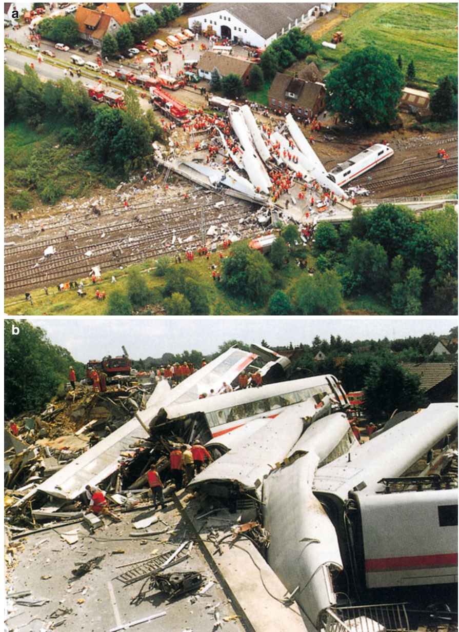
Fig. 2.4 (a, b) The high-speed train incident in Eschede, Germany, in June 1998. An overheated wheel locked and cut the rail off, and the wagons behind it derailed and crashed into a concrete bridge, which collapsed and crushed parts of the train. One hundred one people died and 87 were severely injured. The pictures illustrate the difficult and time-consuming work to rescue many trapped patients (From Hülse and Oestern 1999 with permission)
