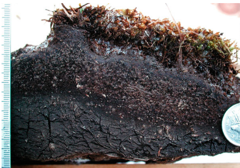
Fig. 2.15 Reticulated vein ice in frozen clay beneath a wetland in Resolute. Note frost crystals in the top moss layer formed by condensation of vapor that fluxed upward from the soil
