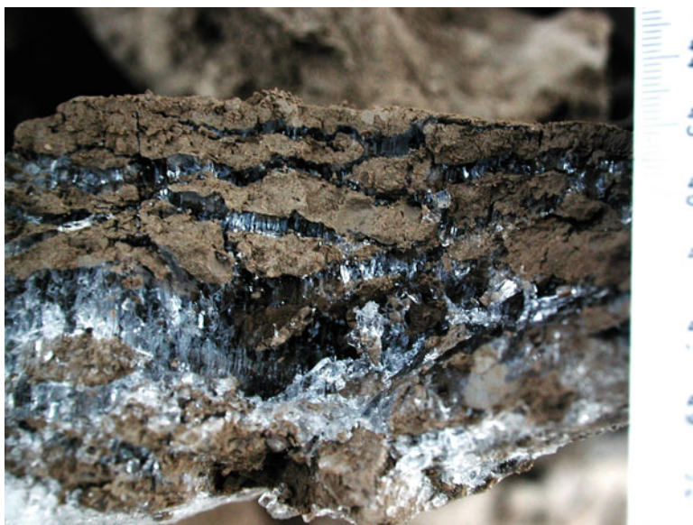
Fig. 2.12 Layers of segregated ice in silty soil, Resolute, with vertical lines of air bubbles in the ice lenses oriented perpendicular to the downward freezing front
