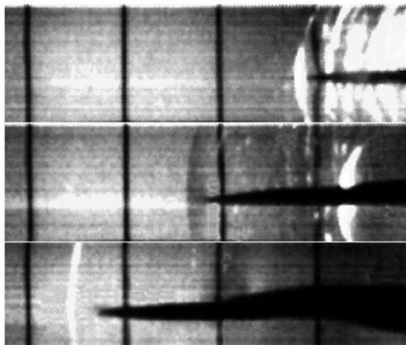
Fig. 6 Record of supersonic motion through water (video frames)
