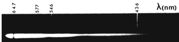
Fig. 2.21 Spectrum of a white light beam after reflection from a gold grating of Fig. 2.20 with groove height 37 nm with incidence 6.6^\circ . Reprinted [50], with permission from Elsevier
