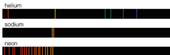
Fig. 2.18 The famous sodium D_1 and D_2 lines, and the D_3 line of helium which was identified by Lockyer and Janssen in the Sun. The conditions in the solar corona allow only for the D_3 line to appear
