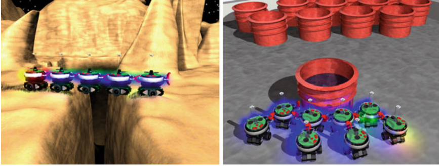
Fig. 2.1 Two examples of robotic entities self-assembled into morphologies appropriate for the task. Left a connected robotic entity crosses a gap. A line formation is well-suited to this task, since it allows the entity to stretch further and minimises the number of robots suspended over the gap. Right robots physically connected in a shovel shape to push a heavy object
