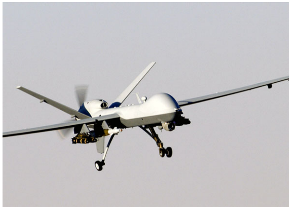
Fig. 2.18 The MQ-9 Reaper is an updated version of the Predator UAS. It is primarily used as a persistent hunter-killer UAS for critical time-sensitive targets and secondarily for intelligence gathering [8] (Photo Credit: US Air Force, Staff Sgt. Brian Ferguson)
