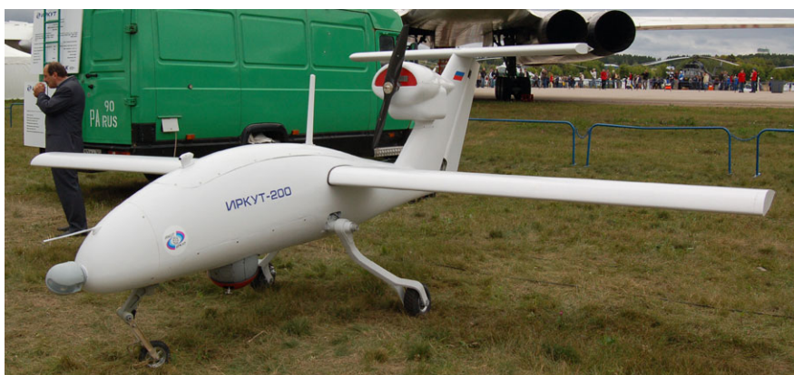
Fig. 2.27 The Irkut-200 Aerial Remote Sensing System with up to 12 hours of flight endurance (Photo Credit: Wikimedia Commons User Allocator)
