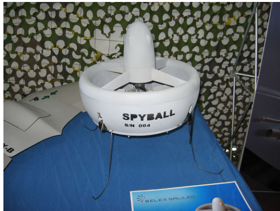
Fig. 2.58 The SELEX Galileo Spyball is an ultra-light UAS that can fit inside a rucksack (Photo Credit: Wikimedia Commons User Causa83)
