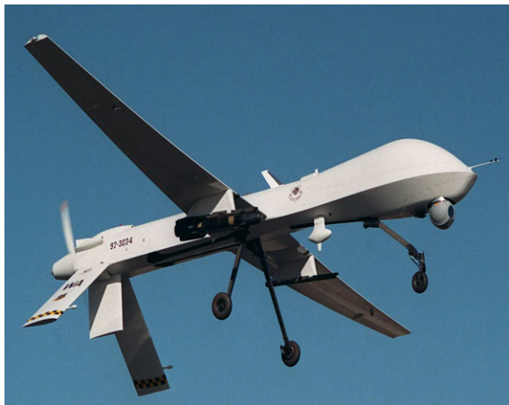
Fig. 2.16 An armed MQ-1 Predator flying a training mission. The MQ-1 is used for armed reconnaissance, airborne surveillance and target acquisition, can carry two laser-guided missiles and employs a crew of two [6] (Photo Credit: US Air Force)
