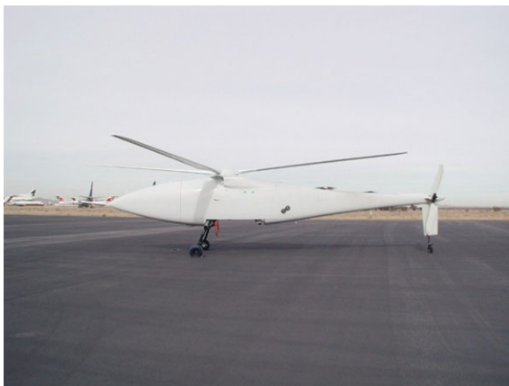
Fig. 2.33 The A-160 Hummingbird built by Boeing/Frontier. It is a demonstrator for improvements in range endurance and controllability [7] (Photo Credit: US DoD)
