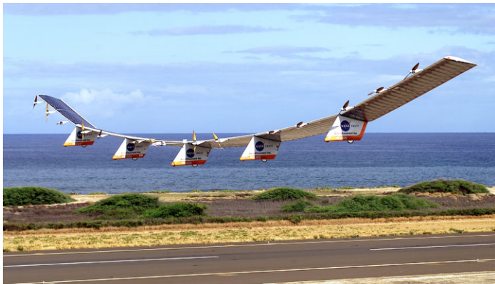
Fig. 2.38 The Helios UAS developed by NASA and AeroVironment. During its second high-altitude flight, it reached 96,863 ft, shattering the existing world altitude record for sustained level flight for both propeller and jet-powered aircraft (Photo Credit: NASA)
