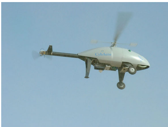
Fig. 2.34 The APID55 is a multi-purpose, fully autonomous helicopter platform with an endurance of over three hours and payload capacity of over 50 kg. It is built by Cybaero (Photo Credit: Cybaero)
