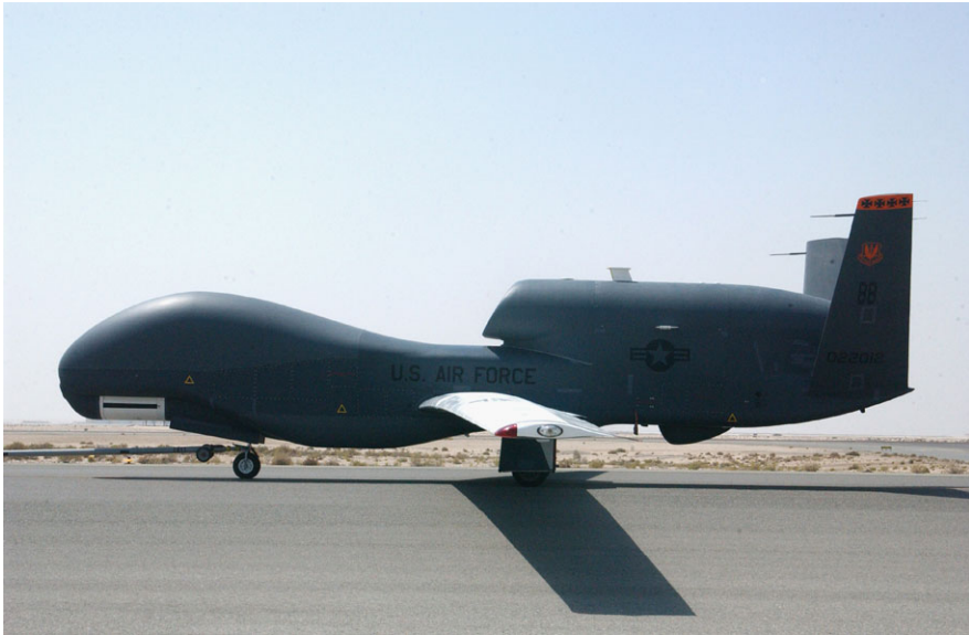
Fig. 2.17 The RQ-4 Global Hawk is a high altitude, long endurance UAS . It was the first UAS to do a trans-pacific crossing [5] (Photo Credit: US Air Force, Master Sgt. Jason Tudor)
