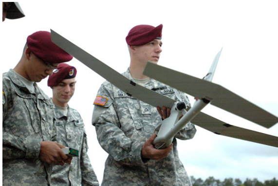
Fig. 2.47 The Raven is a back-packable UAS for “over the hill” and route reconnaissance that evolved from the Pointer UAS. In the photo paratroopers are training with an RQ-11 Raven (Photo Credit: US Army, Sgt. Amanda Jackson)
