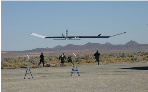
Fig. 2.41 The Zephyr is a solar-powered, high endurance UAS developed by Qinetiq. In July of 2008 it performed an 82 hour long flight (Photo Credit: Qinetiq)
