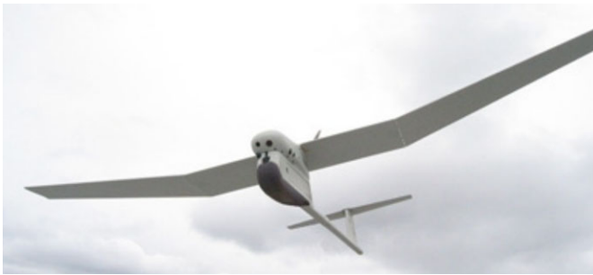
Fig. 2.44 The Puma is another evolution from the Pointer UAS. There are two versions available, the Aqua Puma and the Terra Puma for marine and land environments respectively (Photo Credit: US DoD)
