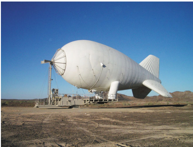
Fig. 2.53 The Persistent Threat Detection System (PTDS) is equipped with a high resolution EO/IR payload used for surveillance (Photo Credit: US Army)
