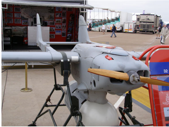
Fig. 2.24 The BAE Systems Phoenix was a British surveillance drone used in Kosovo and Iraq until its retirement (Photo Credit: Wikimedia Commons User BilborneOne)
