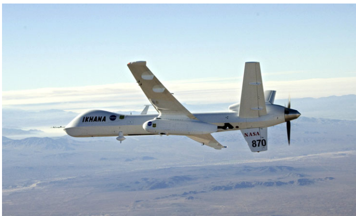
Fig. 2.40 The Ikhana is a Predator B UAS acquired by NASA and retrofitted for earth science missions (Photo Credit: NASA)
