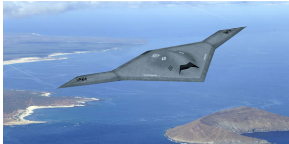
Fig. 2.32 The X-47 started from the DARPA sponsored J-UCAS and is now part of a US Navy program to develop a carrier-based UCAS (Photo Credit: DARPA)
