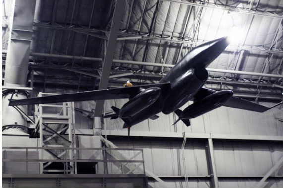
Fig. 2.7 The AQM-34Q, one of several variations of the Ryan Model 147 unmanned reconnaissance drone, used in the 1960's and 1970's (Photo Credit: National Museum of the USAF)
