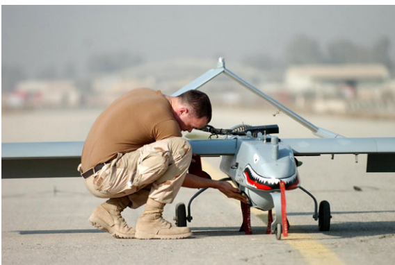
Fig. 2.20 The RQ-7 Shadow is developed by AAI for the US Army and has been deployed in Iraq (Photo Credit: US Army)
