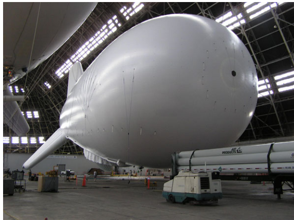
Fig. 2.52 Joint Land Attack Elevated Netted Sensor (JLENS) by Raytheon/TCOM capable of providing over-the-horizon surveillance (Photo Credit: US Army)
