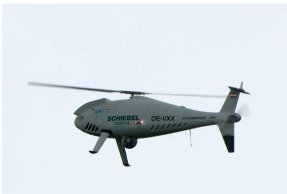
Fig. 2.35 The Schiebel S-100 is a helicopter UAS used by a number of nations particularly for navy operations (Photo Credit: Matthias Kabel)
