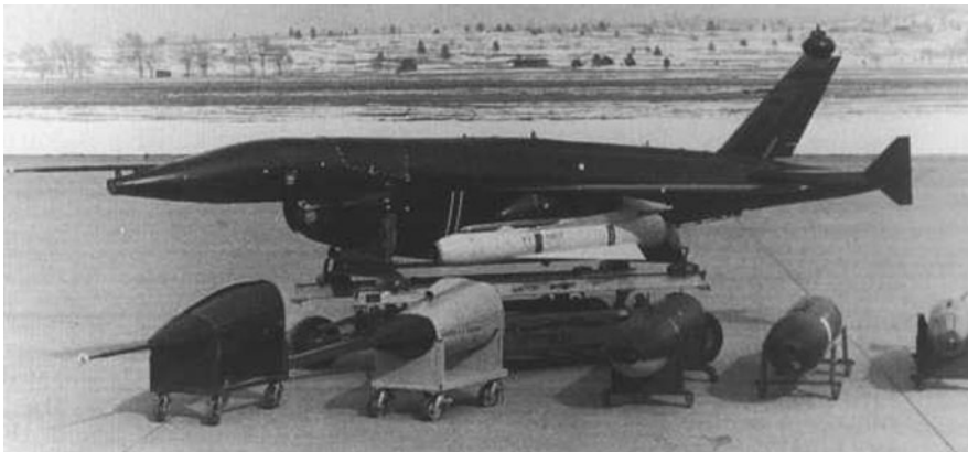
Fig. 2.8 The BGM-34C was another member of the Ryan Model 147 family. It was a multi-role drone capable of performing reconnaissance, electronic counter-measure and strike missions (Photo Credit: US Air Force)
