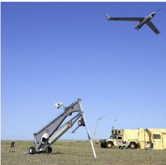
Fig. 2.21 Scan Eagle is a low-cost, long endurance UAS used by the US Marine Corps [7] (Photo Credit: US Air Force)
