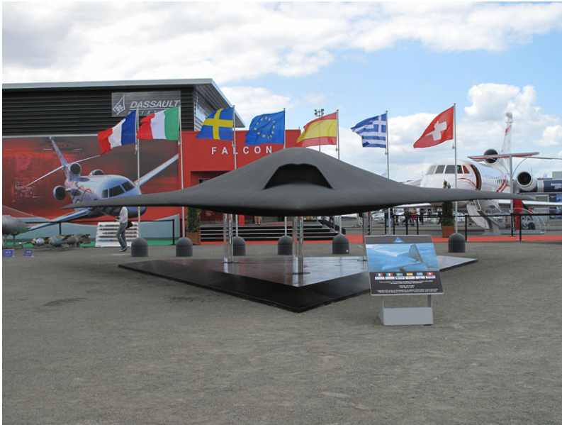
Fig. 2.29 The Neuron is an experimental UCAS being developed by a consortium of European companies (Photo Credit: Wikimedia Commons User Tangopaso)
