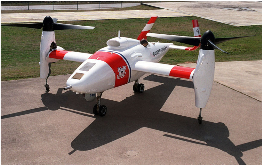
Fig. 2.61 The Eagle Eye is a tilt-rotor UAS developed by Bell Helicopter. It was selected by the US Coast Guard for its Deepwater program but was put on hold in 2007 (Photo Credit: US Coast Guard)
