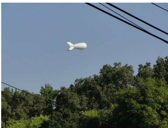
Fig. 2.54 The Rapid Aerostat Initial Deployment (RAID) is a smaller version of the JLENS, used in missions of area surveillance and force protection against small arms, mortar and rocket attacks. (Photo Credit: US Army)
