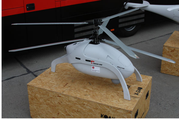
Fig. 2.60 The KOAX X-240 is a Swiss coaxial unmanned helicopter with 90min endurance (Photo Credit: Wikimedia Commons User ILA-boy)
