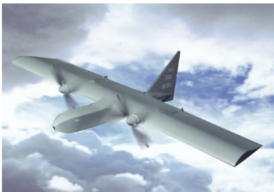
Fig. 2.51 The Dragon Eye is a small UAS used by the US Marine Corps for short-range Surveillance and Reconnaissance (Photo Credit: US DoD)
