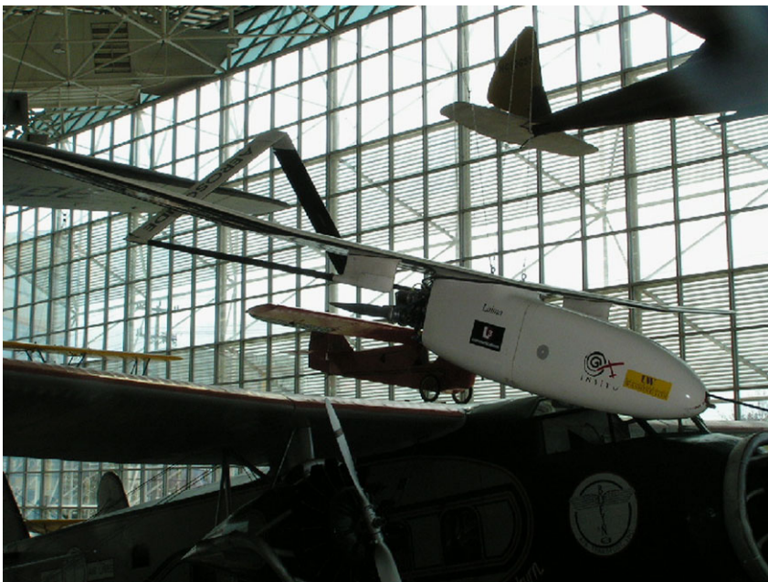
Fig. 2.37 The Aerosonde Laima was the first UAS to make a trans-atlantic crossing [5] (Public domain photo)
