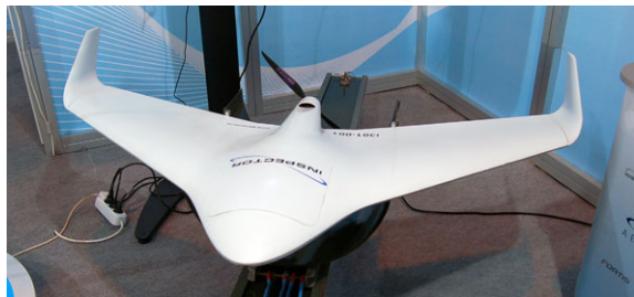
Fig. 2.45 The Aerocon Inspector weighs just 7 kg and has an operational range of 25 km (Photo Credit: Wikimedia Commons User Allocer)
