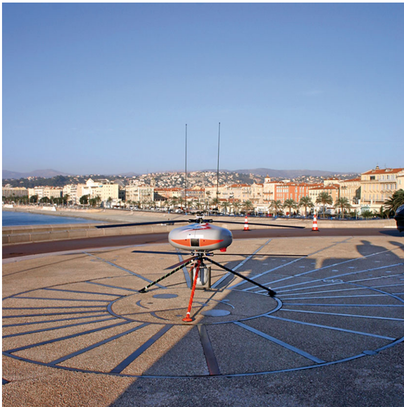
Fig. 2.59 The IT-180 is a French-built light-weight UAS that uses a twin, counter-rotating rotor system (Photo Credit: Infotron)
