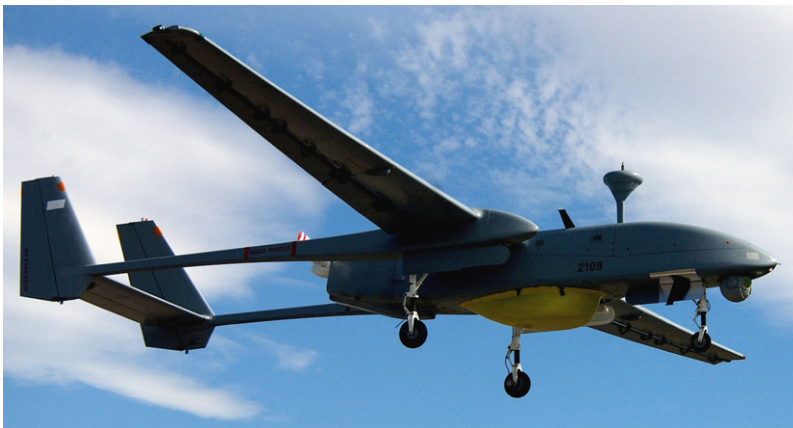
Fig. 2.23 The IAI Heron is medium altitude long endurance UAS. Specifically it can fly for close to two full days. (Photo Credit: US Air Force)
