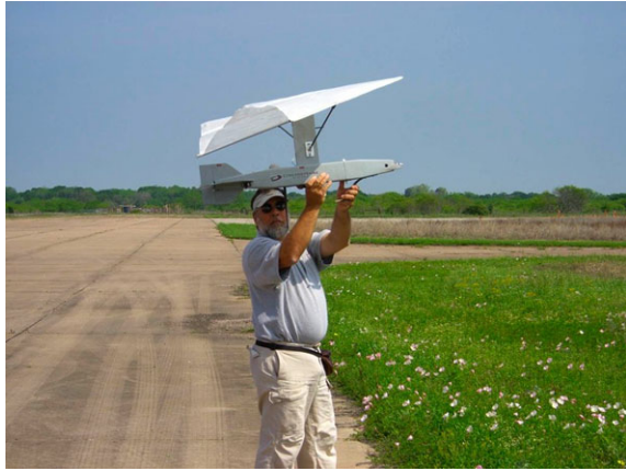
Fig. 2.46 The Cyberbug is a light-weight UAS for urban surveillance applications (Photo Credit: NIST)
