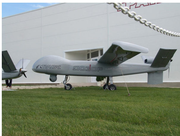
Fig. 2.28 The Dozor-600 is a long endurance surveillance platform similar to MQ-1 Predator or the Hermes 450 (Public domain photo)
