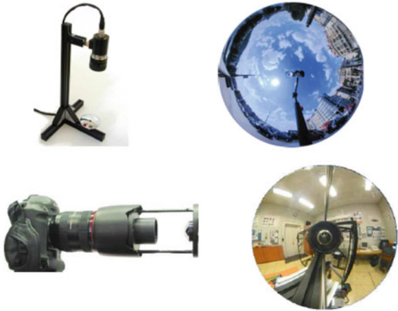
Fig. 2.4 Two configuration of the catadioptric systems and their images
