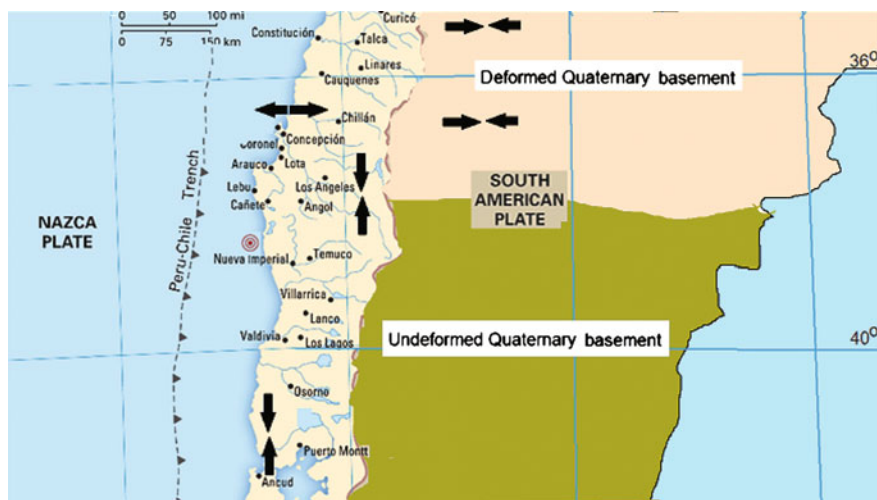
Fig. 2.1 Geological scenario of the 1960 Chile earthquake (bull's eye symbol), after Lavenu et al. (2002). The arrows indicate regions of predominantly compressive or extensional deformation
